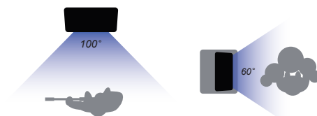
Guitarist Monitor: P15 wedge with 'PS horn' reversed
