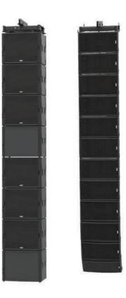
Larger GEO M10 arrays are ideal for live music events with larger audiences. This system flies both main boxes and subs:  $12 \times GEO$  M1012 per side using the Light Bumper and  $8 \times MSUB15s$  with the fourth and eighth sub from the top reversed. One NEXO NUAR rack per side provides power for this stereo system.
