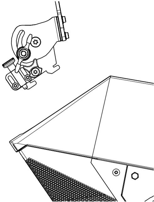
**Positive inclination: locking device towards the back of the cabinet.**
